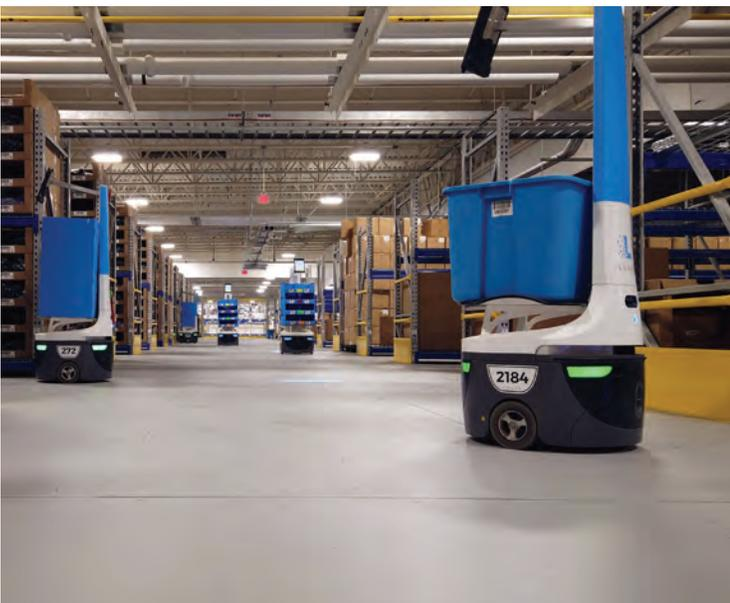
ResinDek with TriGard performance engineered flooring panel provides a level surface for Locus Robotics autonomous mobile robots to navigate quickly and efficiently.
