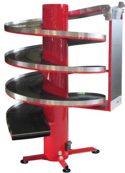
The extended belt of the SVe series consists of multiple parallel belts working together and building a wide belt surface. Working with multiple belts multiplies the belts load capacity and improves the performance while also reducing the radius, resulting in smaller footprints. Overall, it's the optimum mix of features for parcel handling and 24/7 operations such as found in an express delivery service.
