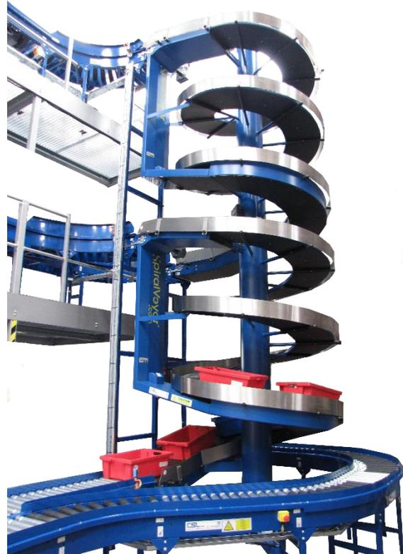
To automate this process engineers stacked two SpiralVeyors on top of each other, creating a multilevel application, where products could be stopped at any level and the direction reversed when needed. Essentially operating as one solution, providing an infeed and outfeed from the first floor and delivering to either the ground or the second floor using the same common conveyors.
